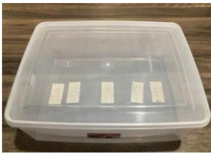
Figure 5. Coal Dust Pollutant Conditioning Box (Fly Ash)
