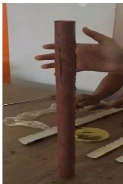
Figure 1. Columns that have come off the mold
